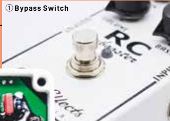
① Bypass Switch
